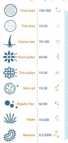
The utility of a filter media is determined by a compromise between micron rate and clogging capacity
